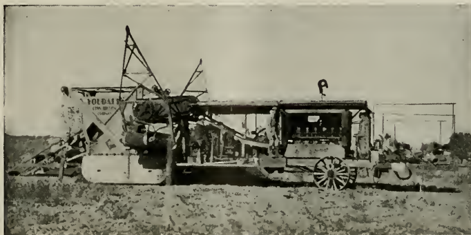
Youdall Construction Company's 120-Ton Buckeye Trencher.
